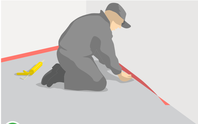
1 Perimeter barrier application
