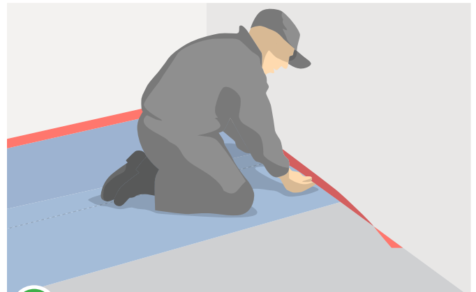
2 Perimeter barrier application
