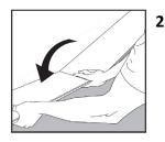
Hold the next plank against the first at an angle to the first one and lay it flat on the floor. Complete the first row in the same way.
