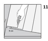
Measure and cut the planks in the last row to the correct size. Allow for a 5mm distance to the wall. No plank should be less than 5cm wide.
